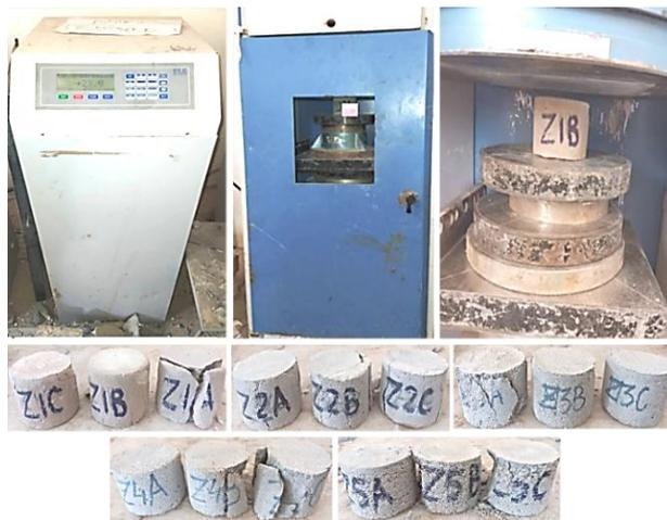
**Fig. (5): Compression Test Machine, Sample under Load and Samples after Failure.**
