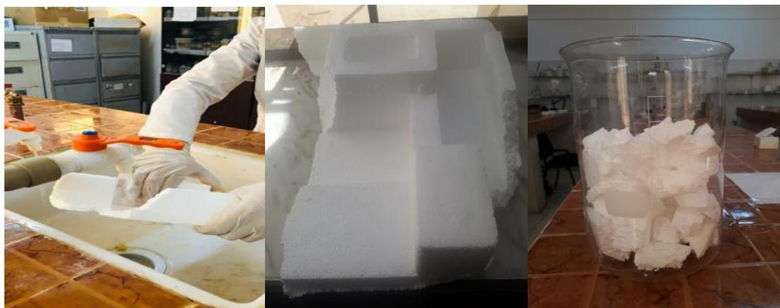
Fig. (4): Preparing a Styrofoam samples for dissolving in organic solvents.
