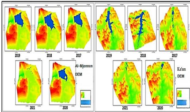
Figure (3): shows a Digital Elevation Model (DEM) of the study area with a spatial resolution of 12.5 meters. DEM data were obtained from the United States Geological Survey (USGS) website.
